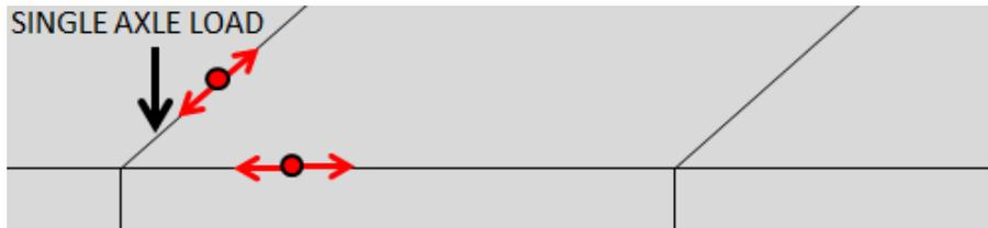
Figure 20: Placement of single axles to determine corner cracking
